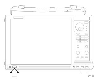
Figure 4: On/Standby switch location
