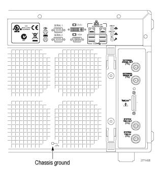
Figure 1: Location of the ground connection on the logic analyzer
