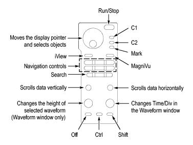
Figure 6: Logic analyzer front panel
