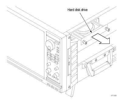
Figure 5: Accessing the replaceable hard disk drive
