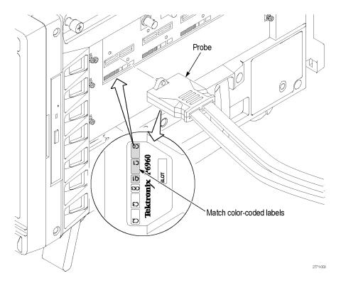
Figure 3: Connecting probes to the logic analyzer
